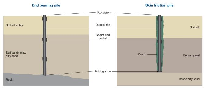
A special grouting shoe gives you the possibility to insert grout material in the annulus between pile and surrounding soil. The driving shoes have to be chosen in accordance with the chosen pile diameter. Two pile diameters are available, 118 mm and 170 mm.
