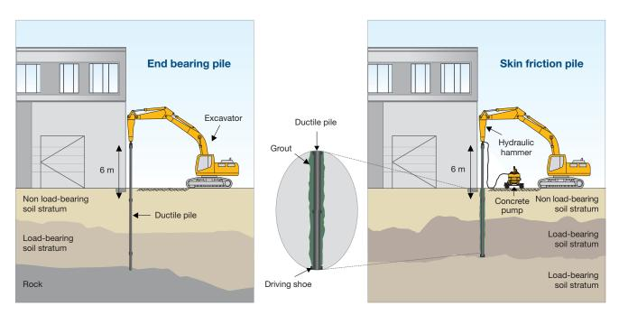
Each 6 m ductile pile section will be driven into the ground and if a pile with
