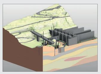
For the Pakal Dul HEP in India, a mighty earth dam is to be filled in a mountain valley. Upstream a cut-off wall is planned in the river sediments of sand and boulder masses down into the unweathered fresh rock. The contact zone between soil and fresh rock is sealed by grouting.
