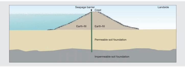
Seepage, piping, partial liquefaction, surface erosion due to flooding or wave action, usually cause significant damage to the protection system. With the appropriate product, such as a cut-off wall, this can be prevented or significantly mitigated.
