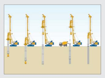
Casing installation with the rotary drive of the drill rig (pushing and rotation).
