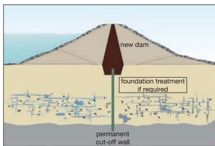
Cut-off wall in operation stage 2
