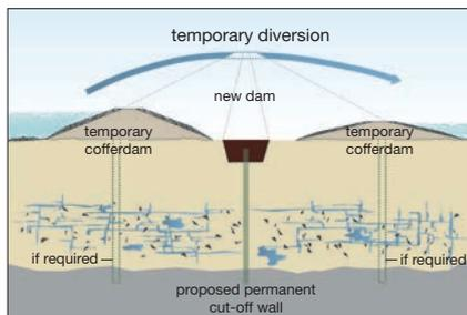
**Cofferdams for New Embankment Dam founded on alluvium**
