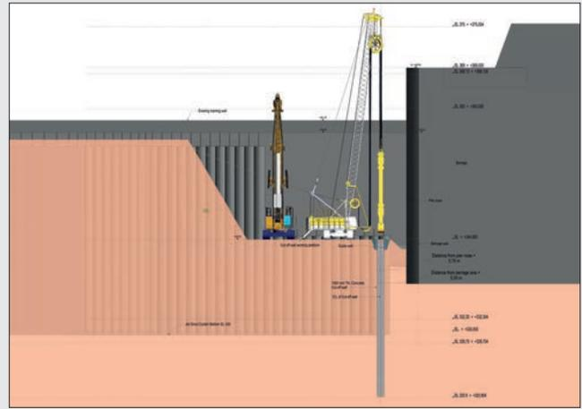
For the Pakal Dul HEP in India, a mighty earth dam is to be filled in a mountain valley. Upstream a cut-off wall is planned in the river sediments of sand and boulder masses down into the unweathered fresh rock. The contact zone between soil and fresh rock is sealed by grouting.
