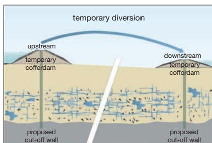
**Cofferdams for excavation pits for New Concrete Dam founded on rock**
