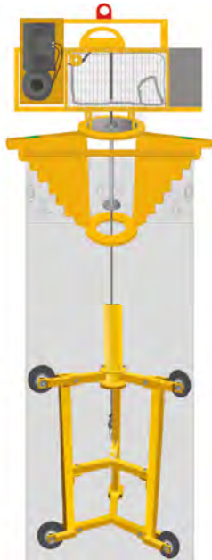
Schematic diagram of the Rope Inclinometer
