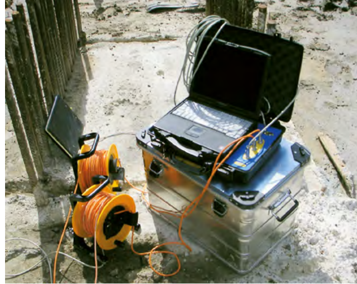
Cross-Hole Ultrasonic Monitor (CHUM) unit set up on site ( www.Piletest.com )
