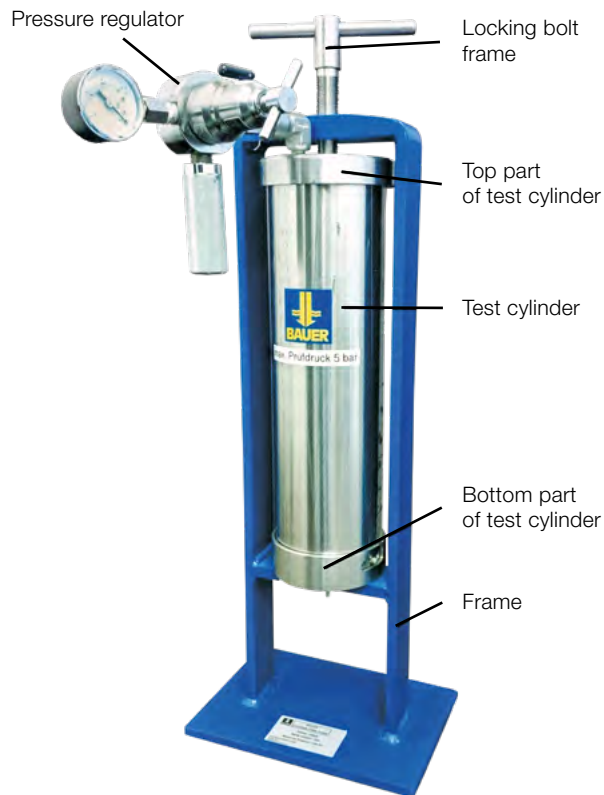
Setup BAUER Concrete Filter Press
