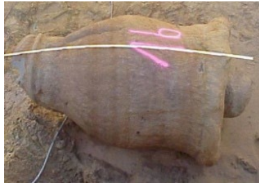
Fig. 7. Jet grout column produced in interbedded soil layers
