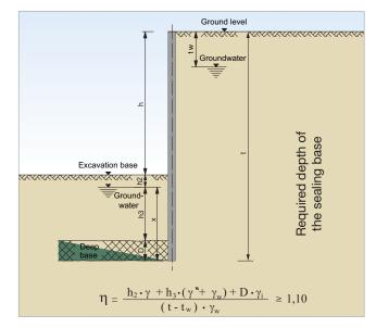
plane of the blanket are set against the forces from the soil and groundwater acting above the blanket.
