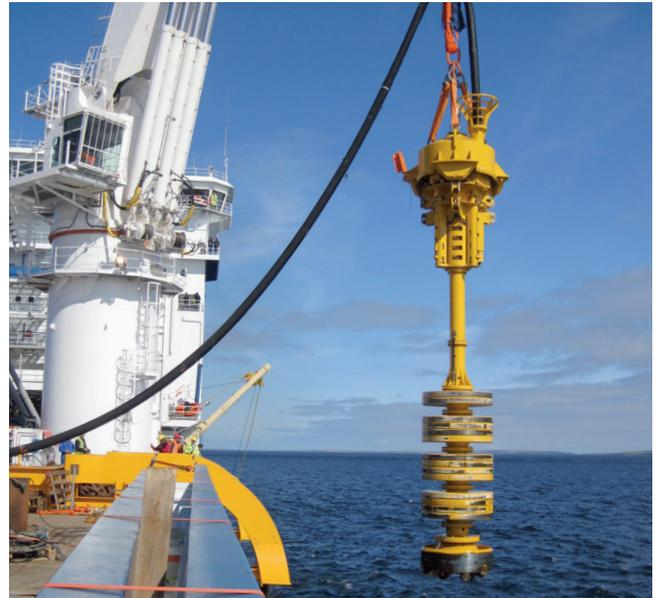
*BAUER BSD 3000 Seabed Drilling Rig operating the drilling template:*
