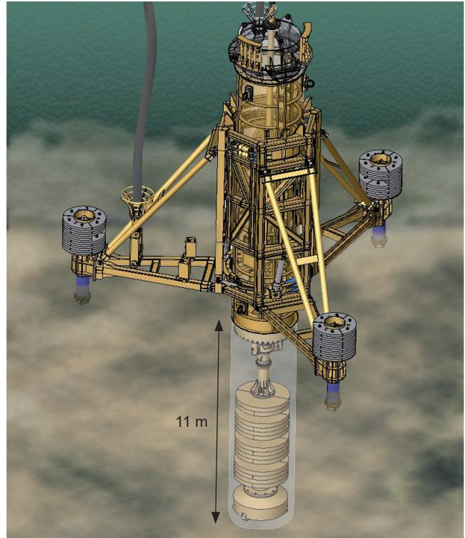
Rock Drilling Uncased with a Template
