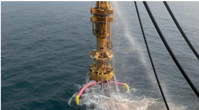
Bauer Dive Drill Seabed Drilling Rig
