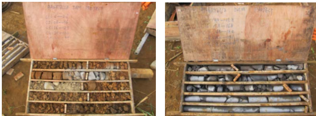
Figure 2 Core boxes showing weathered basalt with some cobbles (left) and fresh competent basalt (right)
